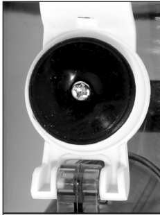
Seal at the closing cap
